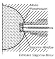
The probe will withstand continuous operation at up to 1000°F and 60,000 psi. All probes are configured to fit the standard 1/2"-20UNF mounting holes used in extruders. SMA fiber optic connectors allow direct connection to spectrophotometers.
